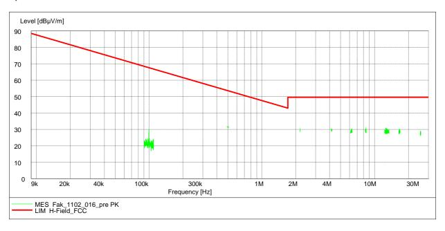
Antenna position 0° EUT position front side
