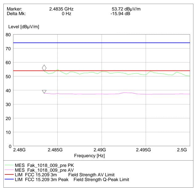
Radiated measurement (higher band edge)
