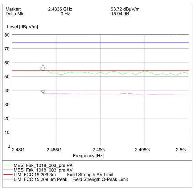
Radiated measurement (higher band edge)
