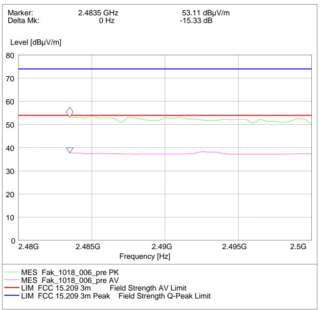
Radiated measurement (higher band edge)
