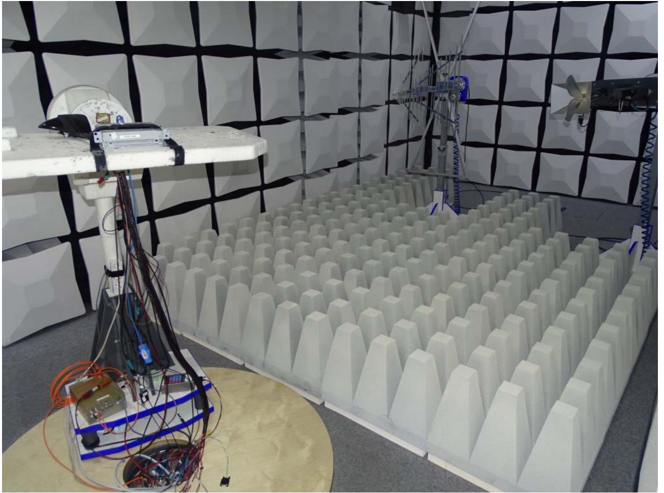
Photo 5: Test setup for radiated measurements in fully-anechoic chamber above 1 GHz
