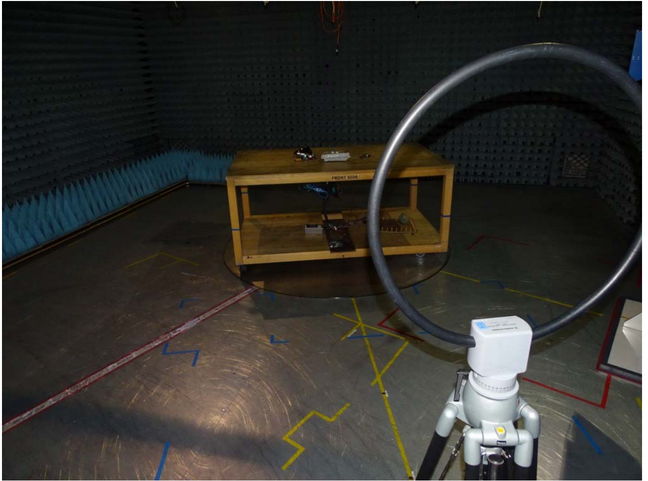
Photo 2: Test setup for radiated measurements below 30 MHz
