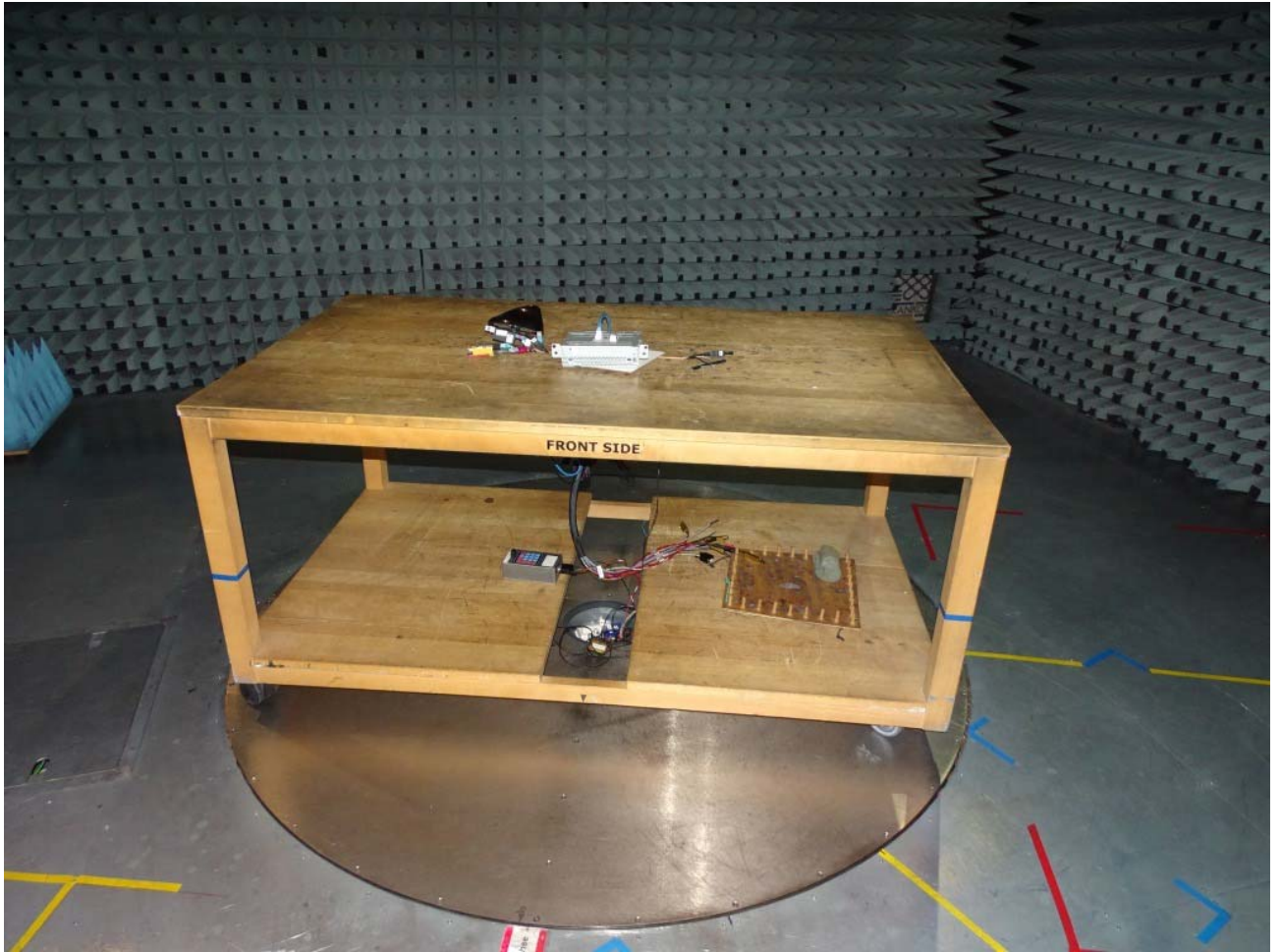
Photo 4: Test setup for radiated measurements in semi-anechoic chamber, front side view
