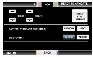
You will not be able to adjust the time until it has been received from the GPS module. Once the time appears, the following settings are available:
