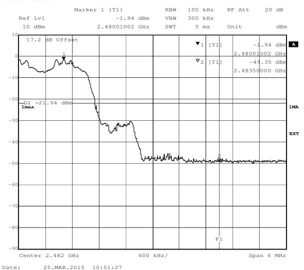
Test: 15c.6; Frequency = hopping, Mode = BT transmit using 3 Mbps with 8DPSK modulation, Method = conducted, band edge = 2400 MHz
