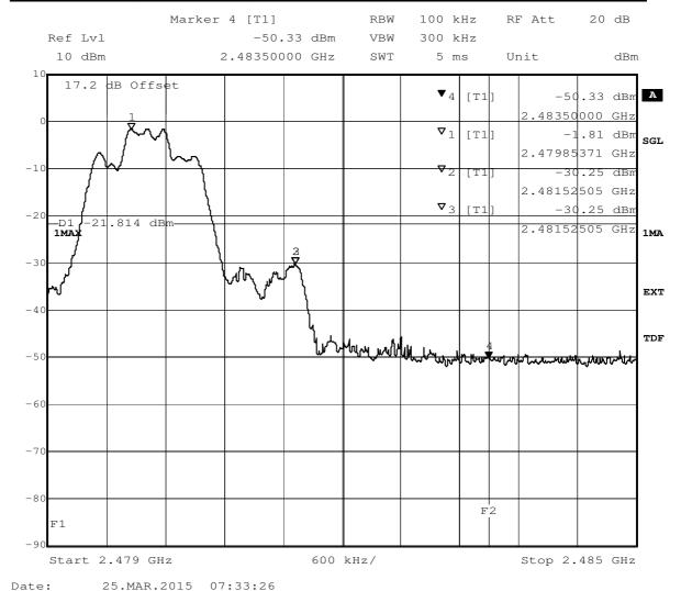
Test: 15c.6; Frequency = 2480, Mode = BT transmit using 2 Mbps with PI/4 DQPSK modulation, Method = radiated
