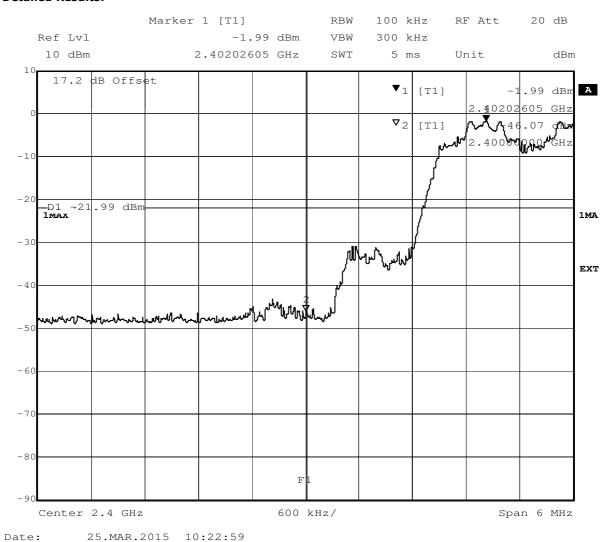
Test: 15c.6; Frequency = hopping, Mode = BT transmit using 3 Mbps with 8DPSK modulation, Method = conducted, band edge = 2483.5 MHz
