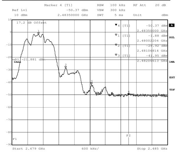
Test: 15c.6; Frequency = 2480, Mode = BT transmit using 3 Mbps with 8DPSK modulation, Method = radiated
