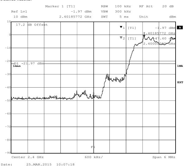
Test: 15c.6; Frequency = hopping, Mode = BT transmit using 2 Mbps with PI/4 DQPSK modulation, Method=conducted, band edge=2483.5 MHz
