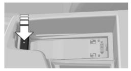
Insert snap-in adapter at the front, arrow 1, and press to the bottom, arrow 2, until the adapter engages.
