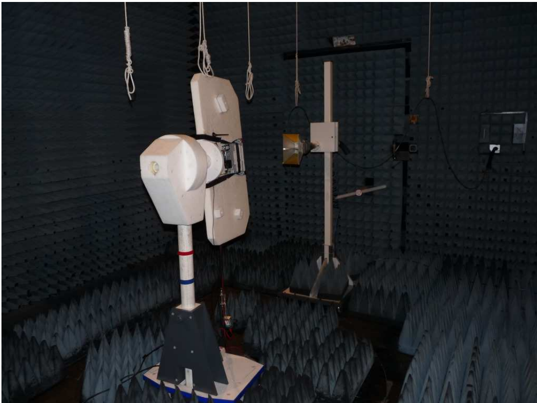
Photo 3: Test setup for radiated measurements (above 1 GHz)
