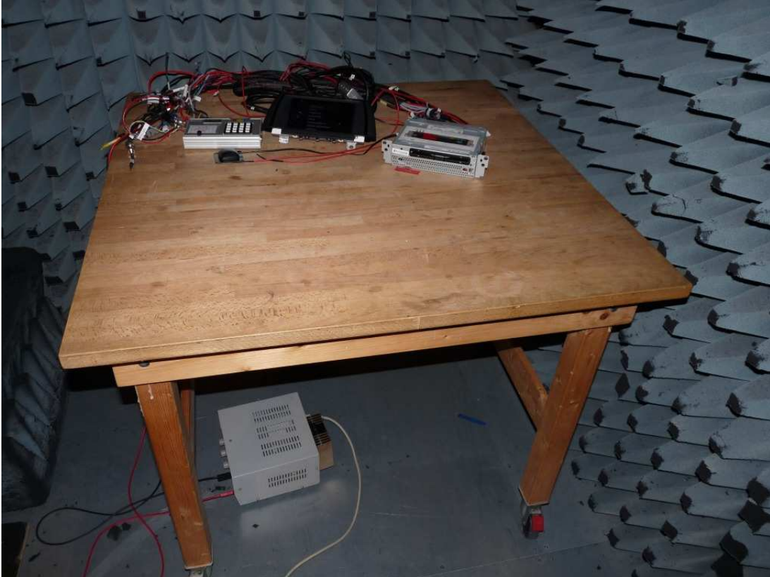
Photo 1: Test setup for radiated measurements (below 30 MHz)
