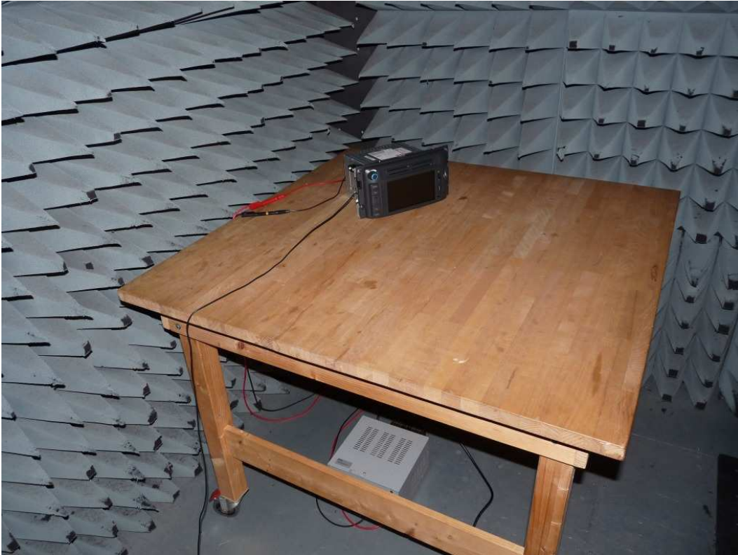
Photo 1: Setup for radiated measurements below 30 MHz
