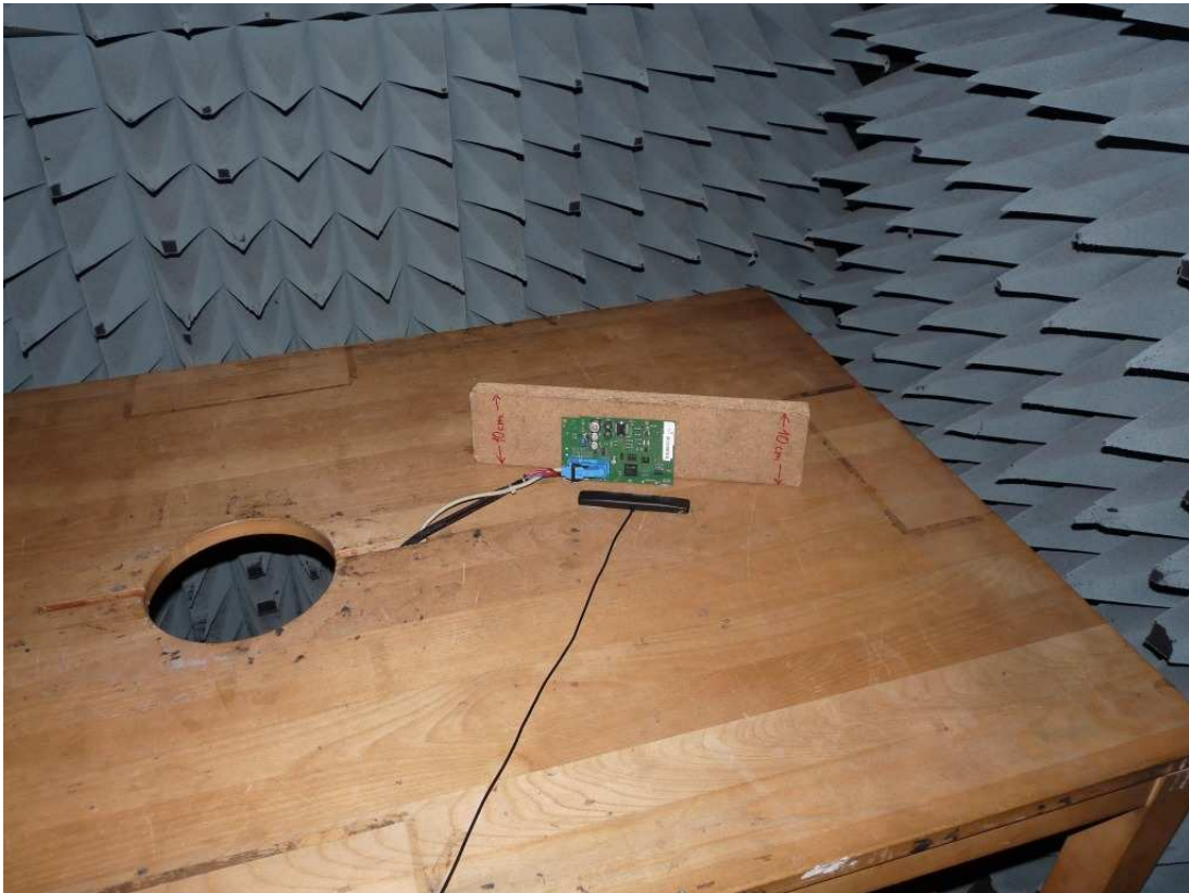
Photo 1: Setup for radiated measurements below 30 MHz
