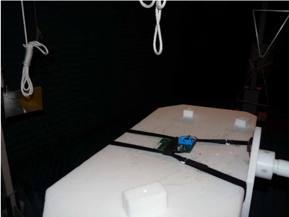
Photo 3: Setup for radiated measurements above 1 GHz
