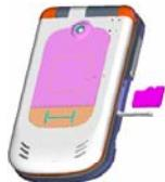
(3) Push T-card gently until it is fixed in the T-card slot and replace the card protective cover. It shows as the below figure:
