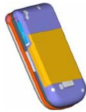
(4) Make sure the golden contact of battery face into the corresponding contact of the phone, and then push down the bottom of battery until it is fixed in the battery slot. At last, replace the battery cover, shown as the below figure
