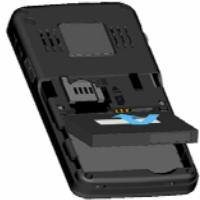
(5) Make sure the battery has been installed correctly, and then slide the battery cover in the direction of the top of the phone until it is covered, as shown below:
