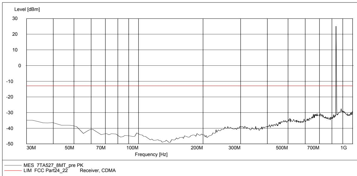
**A.2.3.3 RADIATED SPURIOUS EMISSIONS-Channel 251: 30MHz – 1GHz**
