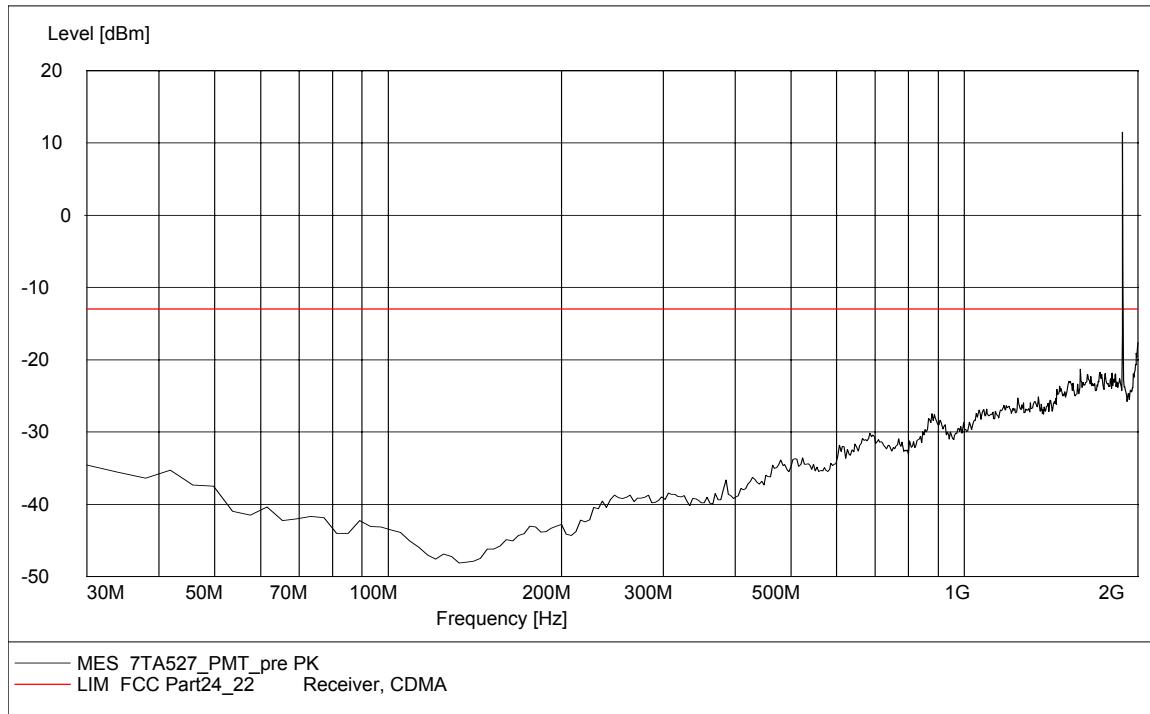
**A.2.3.11 RADIATED SPURIOUS EMISSIONS-Channel 810: 30MHz – 2GHz**
