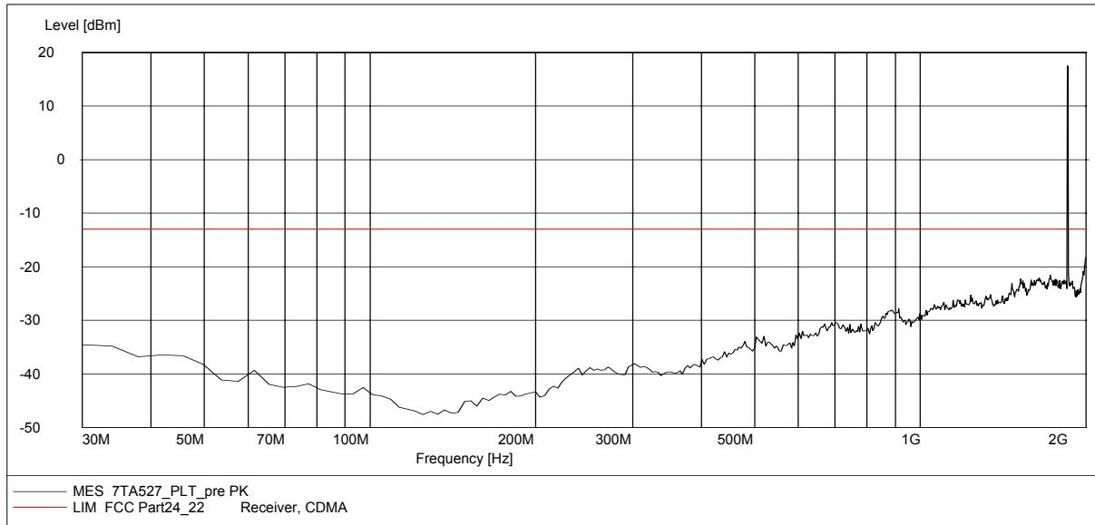
**A.2.3.10 RADIATED SPURIOUS EMISSIONS-Channel 661: 30MHz – 2GHz**
