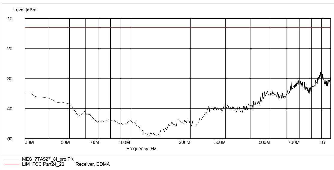
**A.2.3.8 RADIATED SPURIOUS EMISSIONS-EUT in Idle Mode: 1GHz – 10GHz**
