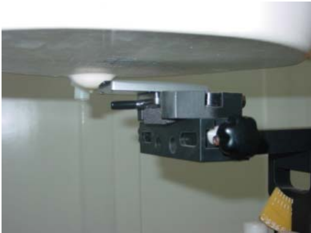
Picture 6 Flat Phantom -- Body-worn Position (toward phantom, the distance from handset to the bottom of the Phantom is 1.5cm)
