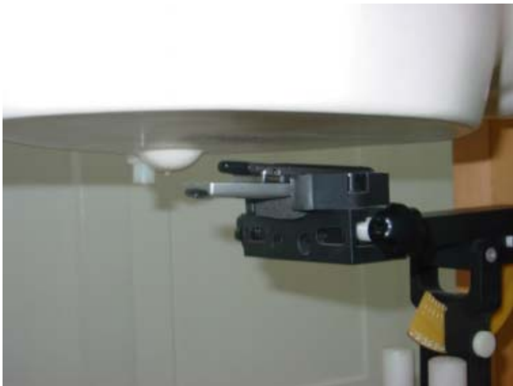
Picture 7 Flat Phantom -- Body-worn Position (toward ground, the distance from handset to the bottom of the Phantom is 1.5cm)
