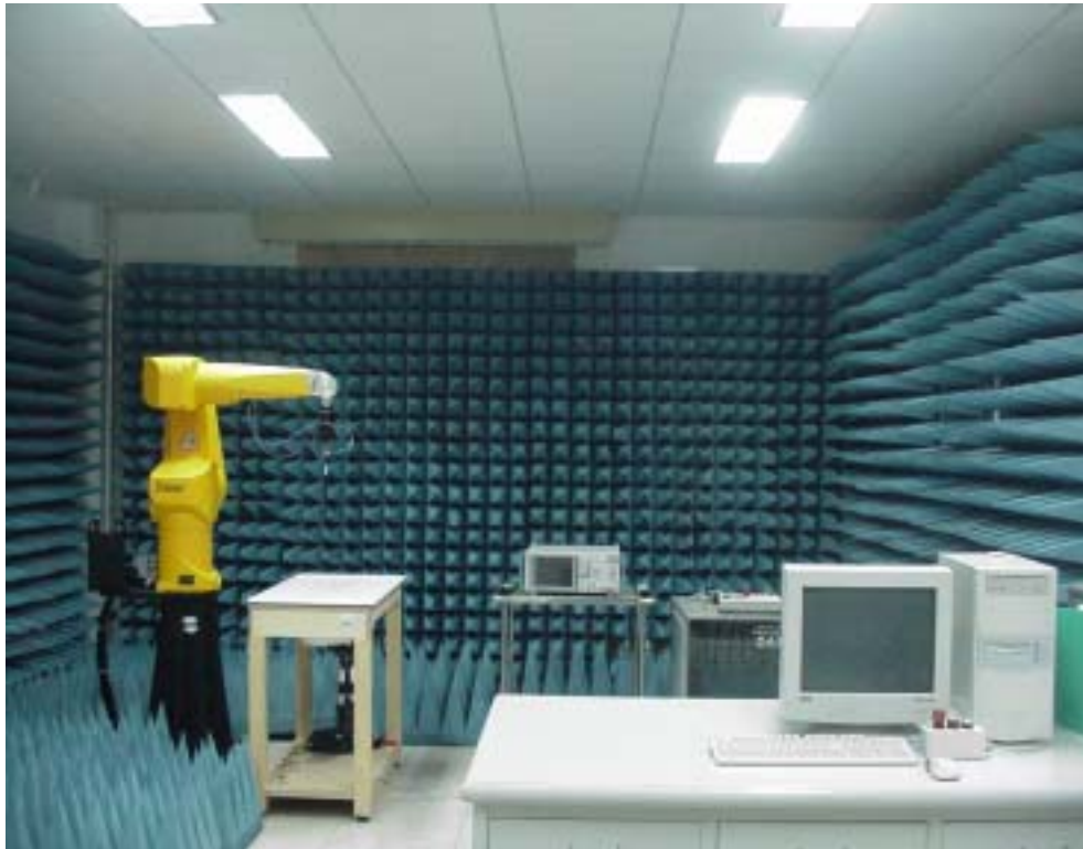
Picture 1 Specific Absorption Rate Test Layout
