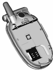
4. Insert the SIM card ensuring that the cut corner is at the top right and the gold contacts of the card face into the phone.
