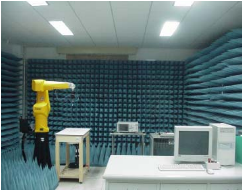
Picture 1 Specific Absorption Rate Test Layout
