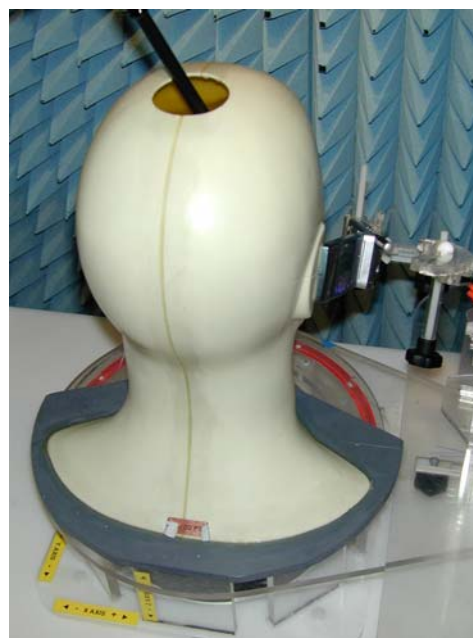
Figure 38. Positional photograph of Amoi DA6 Handset in the Right-hand 15 Degree Position
