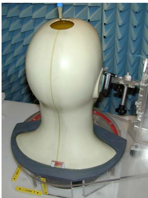
Figure 37. Positional photograph of Amoi DA6 Handset in the Right-hand Cheek Position
