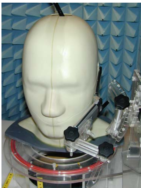
Figure 35. Positional photograph of the Amoi DA6 Handset in the left-hand Cheek Position
