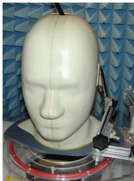
Figure 36. Positional photograph of Amoi DA6 Handset in the Left-hand 15 Degree Position
