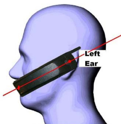
Figure 14. – Side View of Mobile next to head showing alignment.
