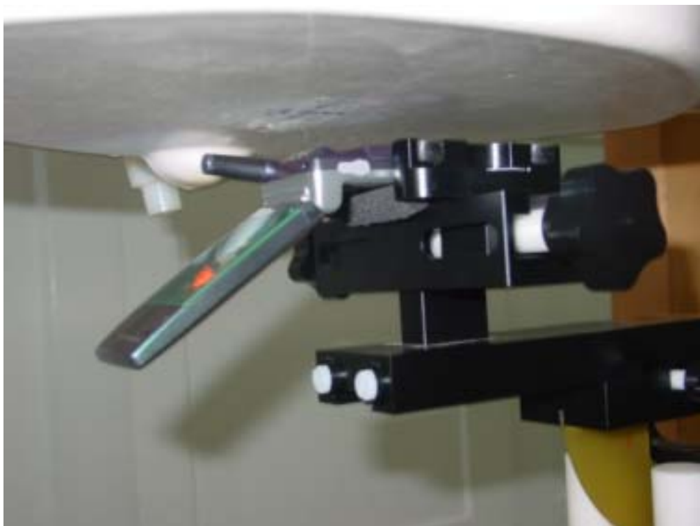
Picture 2 Flat Phantom -- Body-worn Position (toward ground, the distance from handset to the bottom of the Phantom is 1.5cm)
