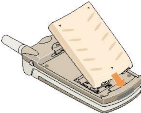
? Push the battery down until it clicks into place. Make sure that the battery is properly installed before switching on the phone.
