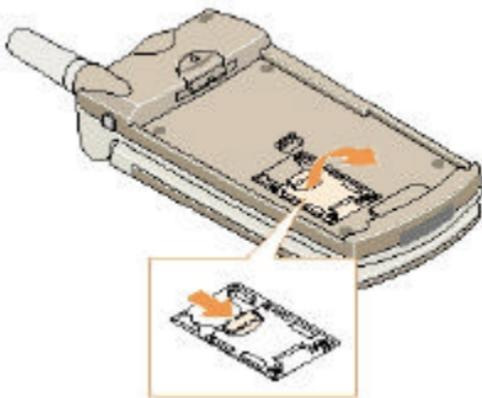
4. Insert the SIM card ensuring that the cut corner is at the top left and the gold contacts of the card face into the phone.
