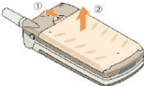
3. Slide the ivory lock in the SIM cardholder as shown below to unlock the SIM card holder and lift it up.
