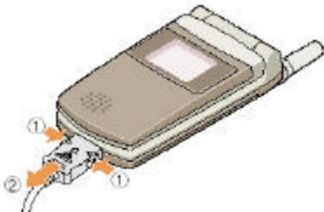
*Note: When disconnect the lead of the adapter from the phone, you should press the buttons on both sides of it, otherwise it's easily damaged.*
