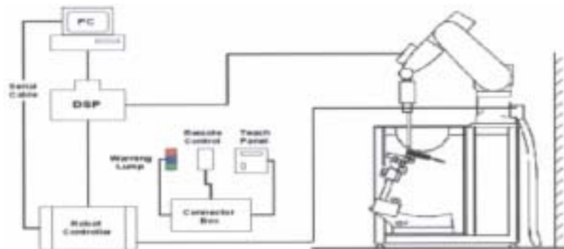
Figure2. SAR Lab Test Measurement Set-up
