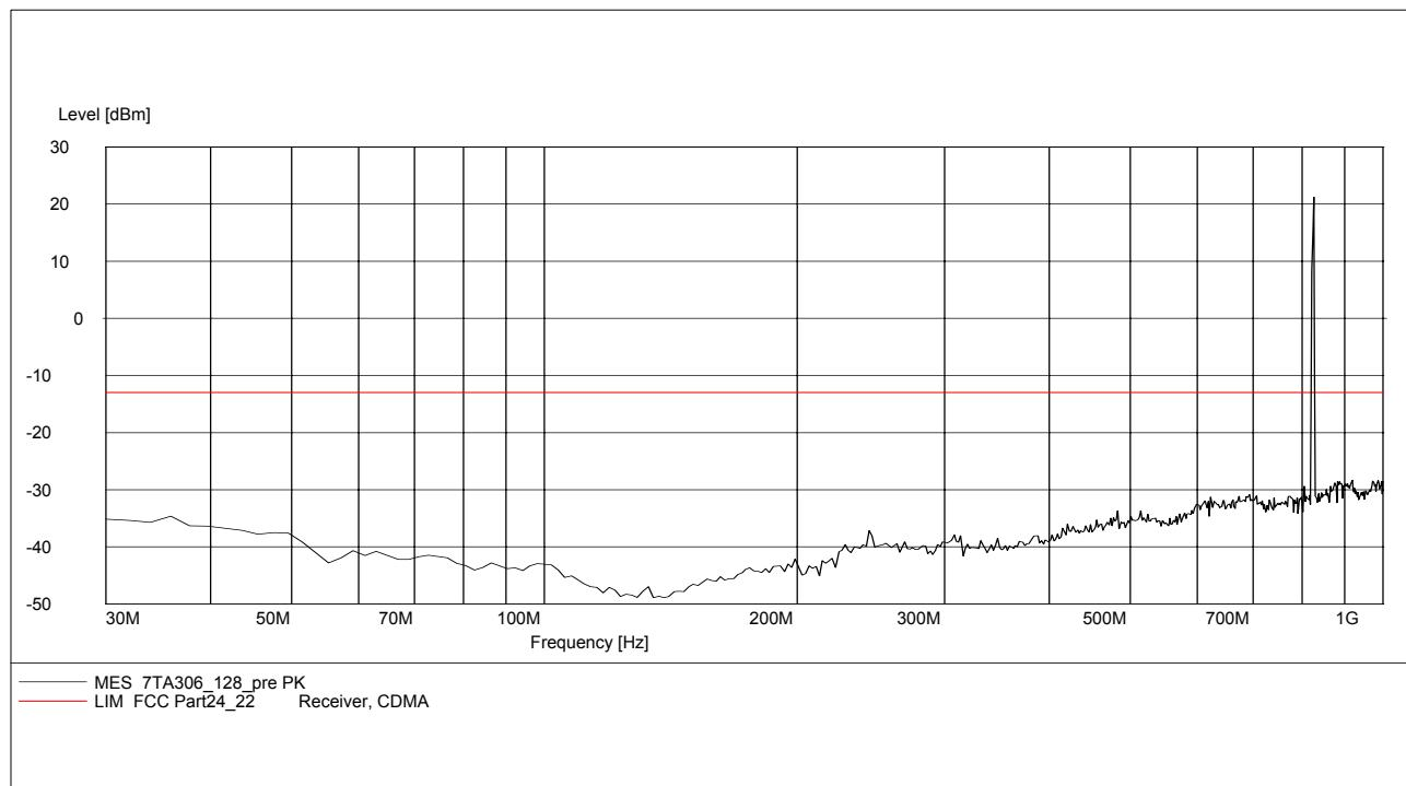
**A.2.3.2 RADIATED SPURIOUS EMISSIONS-Channel 190: 30MHz – 1GHz**
