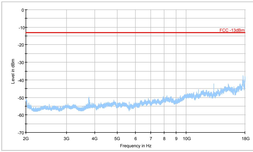
**A.2.3.14 RADIATED SPURIOUS EMISSIONS-Channel 810: 2GHz – 18GHz**
