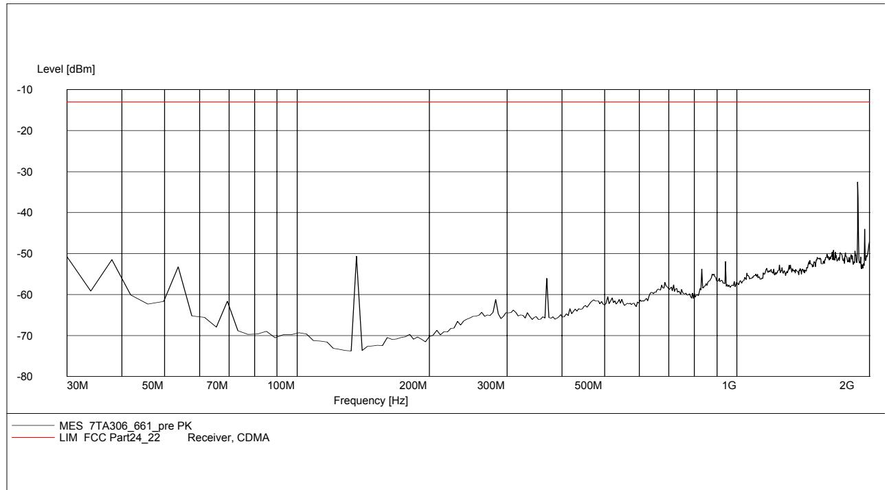
**A.2.3.11 RADIATED SPURIOUS EMISSIONS-Channel 810: 30MHz – 2GHz**
