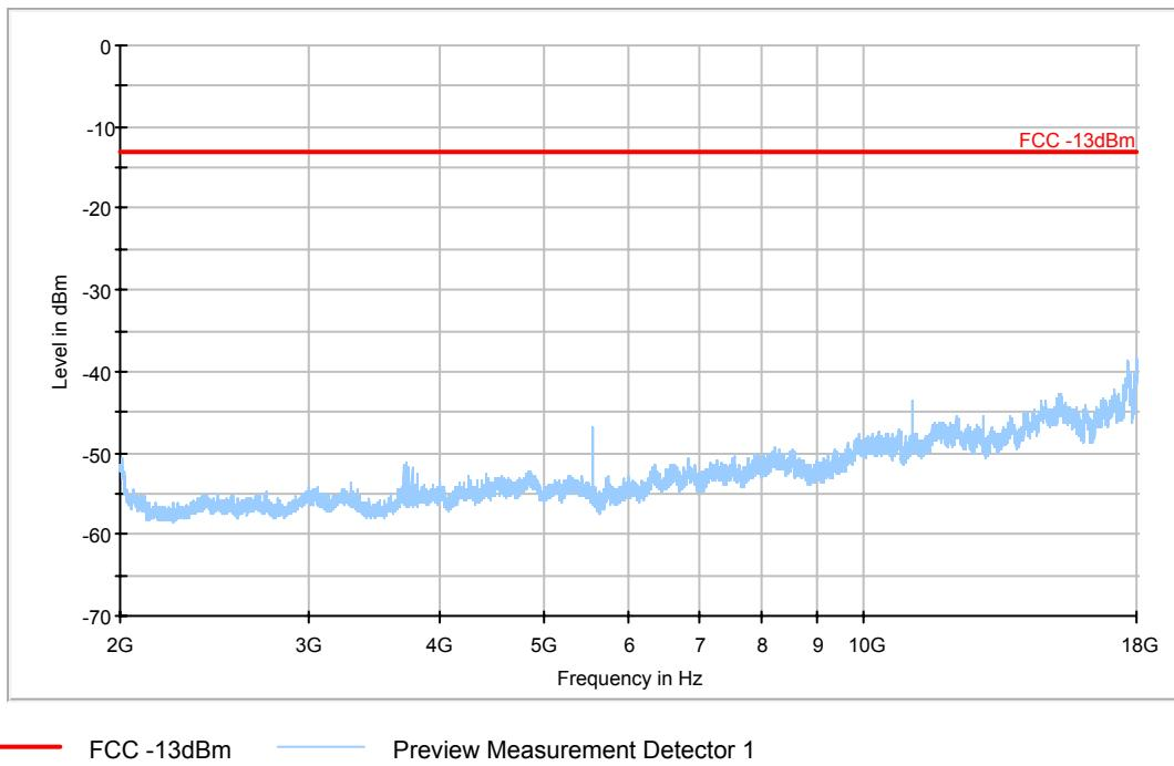
**A2.3.13 RADIATED SPURIOUS EMISSIONS-Channel 661: 2GHz – 18GHz**
