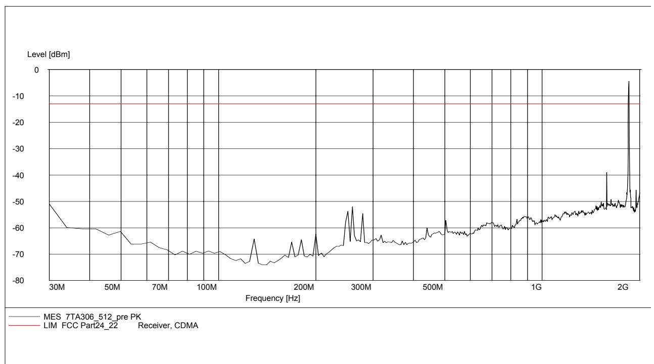
**A.2.3.10 RADIATED SPURIOUS EMISSIONS-Channel 661: 30MHz – 2GHz**
