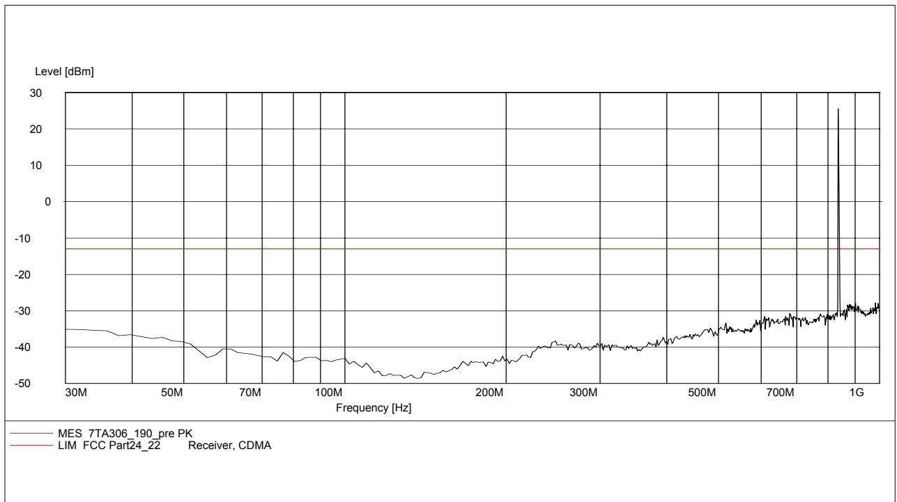
**A.2.3.3 RADIATED SPURIOUS EMISSIONS-Channel 251: 30MHz – 1GHz**
