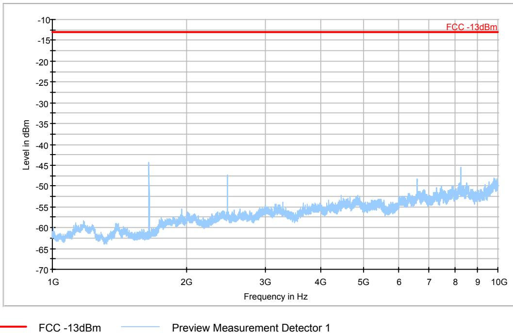
**A.2.3.5 RADIATED SPURIOUS EMISSIONS-Channel 190: 1GHz – 10GHz**
