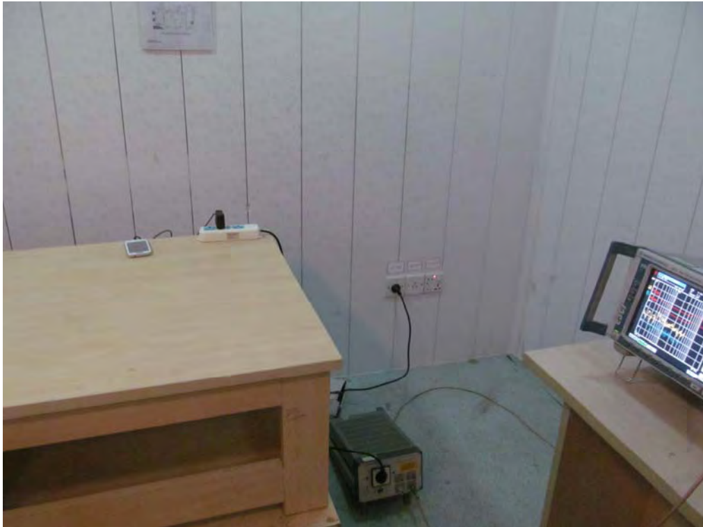
FCC RADIATED EMISSION TEST SETUP
