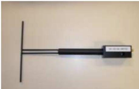
Figure 1 – Satimo COMOSAR Validation Dipole
