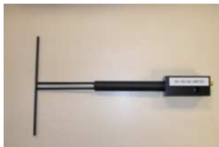
Figure 1 – Satimo COMOSAR Validation Dipole
