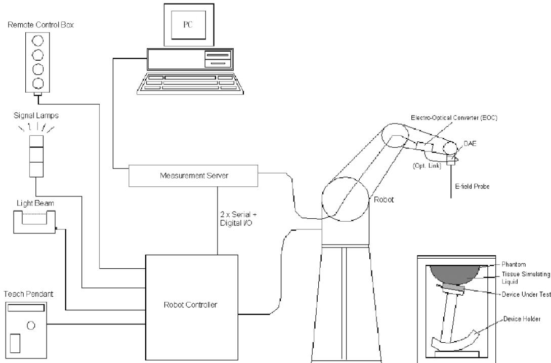
The COMOSAR system for performing compliance tests consists of the following items:
