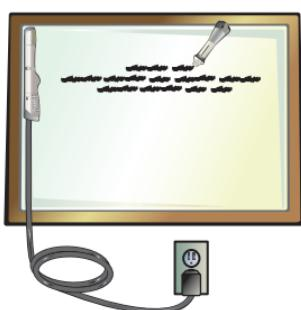
Power on mimio Xi. mimio Xi can be powered by 4 AA batteries or the included AC Adapter.
