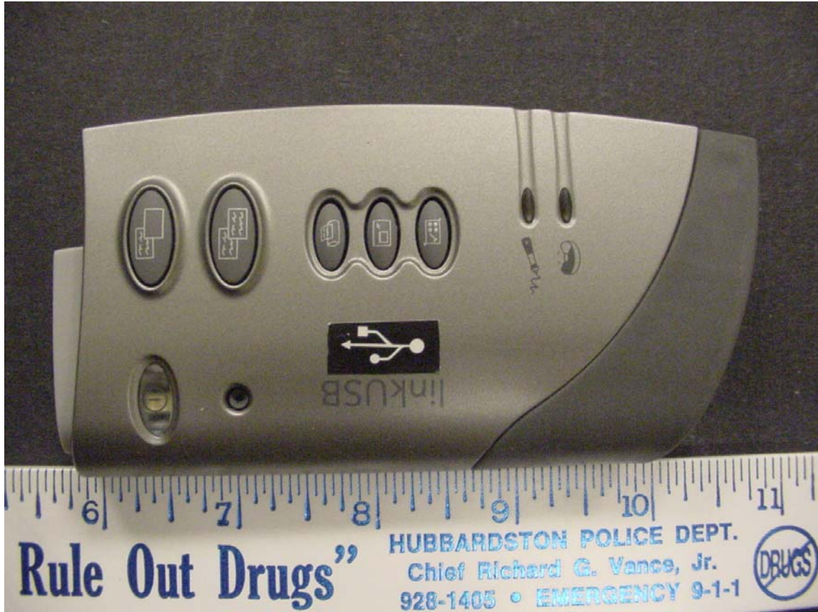
Front of EUT as it appears when removed from the wand.
