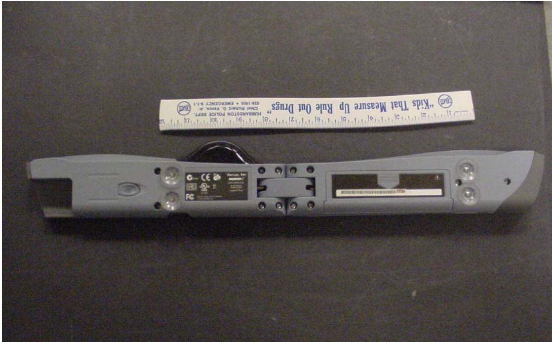
Rear view of EUT and its host, EUT is at the left end of the photo and is removed from the wand by pressing the indent.
