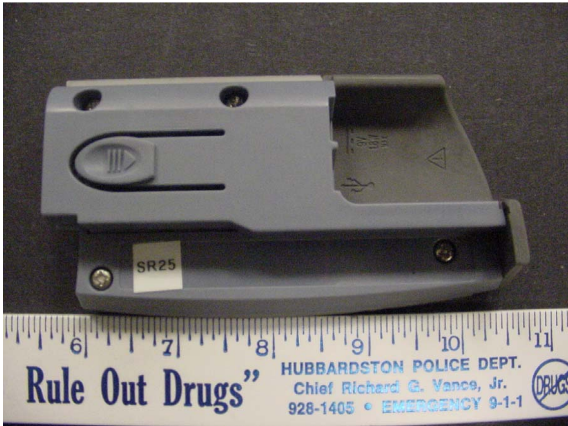
Rear of EUT as it appears when removed from the wand. The inset area where the "SR25" label is located is the location for the FCC and IC ID label.
