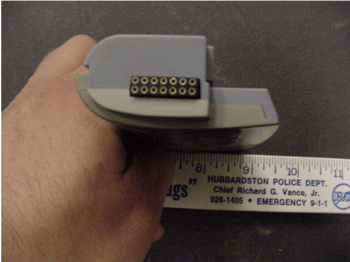
End view of EUT, shows the connector for wand communications and power.
