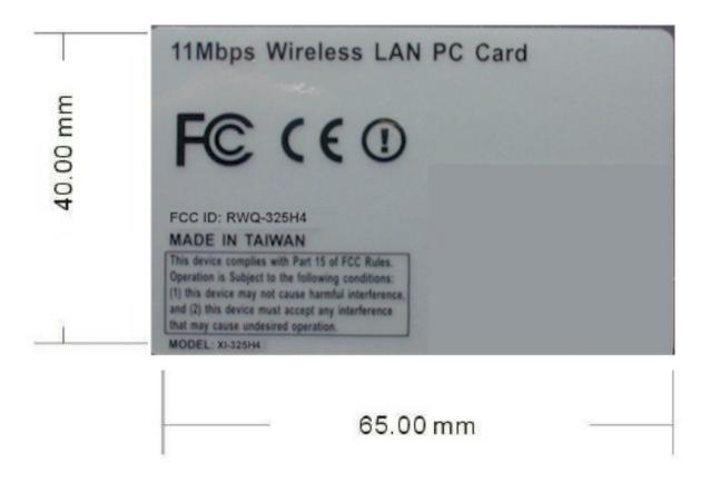
Label Location - Label will be attached directly to the PC Card
