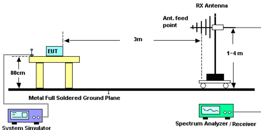
For radiated test above 1GHz
