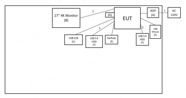
Radiated Emissions Test
