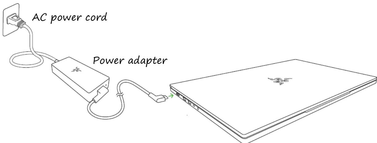
! Use the appropriate power cord for your region. For first time use, please fully charge your laptop first or make sure to connect it to a power outlet before turning it on. It takes at least 2 hours to fully charge your Razer Blade 15.
