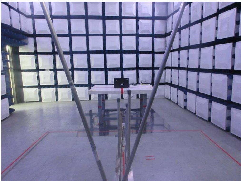
**Radiated Emissions Test Photos****Above 1 GHz**
