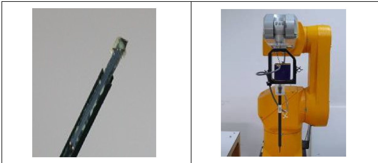
EX3DV4 E-field Probe
