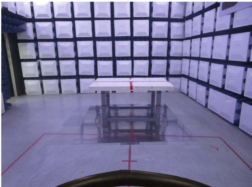
**Radiated Emissions Test Photos****30 MHz to 1000 MHz**
