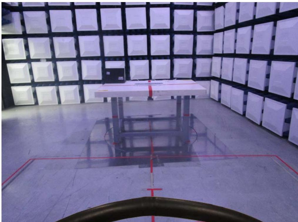
**Radiated Emissions Test Photos****30 MHz to 1000 MHz**
