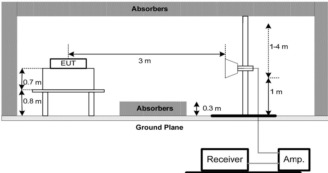
(C) For radiated emissions below 30MHz
