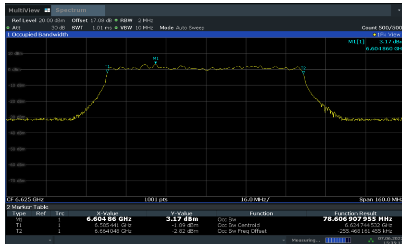
Fig.102 99% Occupied Bandwidth (802. 11ax-HE80, 6625MHz)
