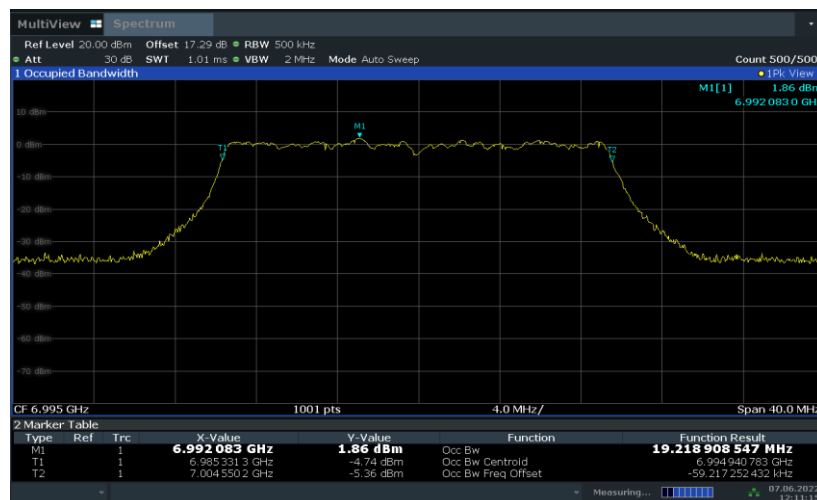
Fig.81 99% Occupied Bandwidth (802.11ax-HE20, 6895MHz)
