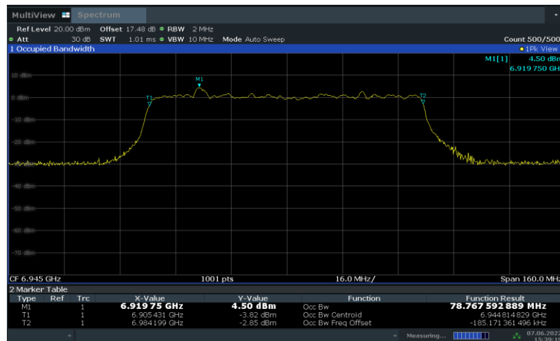
Fig.105 99% Occupied Bandwidth (802. 11ax-HE80, 6865MHz)
