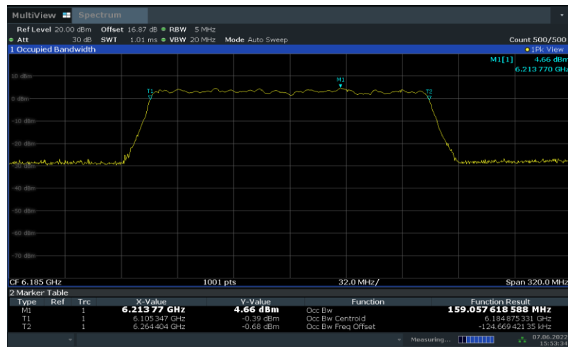
Fig.108 99% Occupied Bandwidth (802. 11ax-HE160, 6025MHz)
