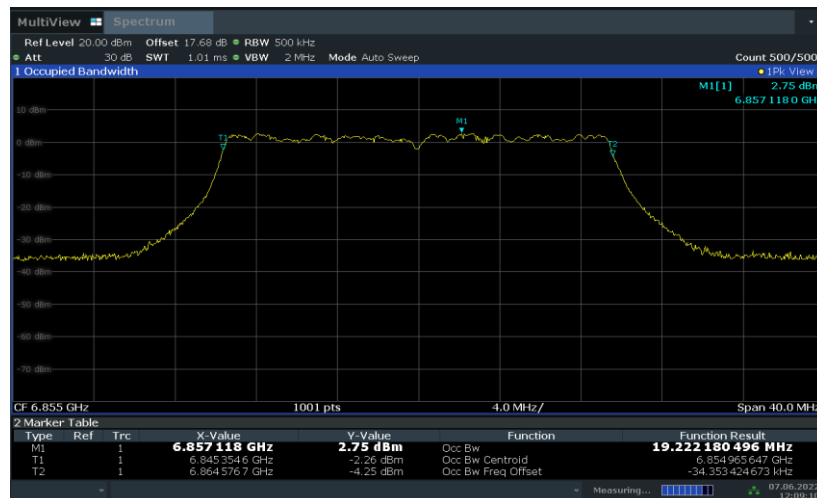
Fig.78 99% Occupied Bandwidth (802.11ax-HE20, 6695MHz)
