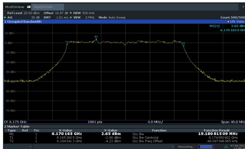
Fig.72 99% Occupied Bandwidth (802.11ax-HE20, 6175MHz)
