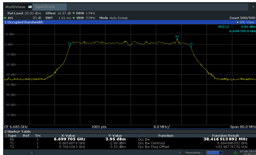
Fig.90 99% Occupied Bandwidth (802.11ax-HE40, 6565MHz)
