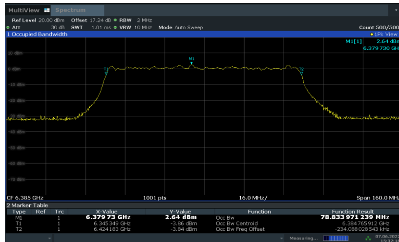
Fig.99 99% Occupied Bandwidth (802. 11ax-HE80, 6385MHz)
