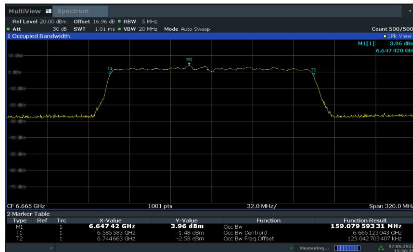
Fig.111 99% Occupied Bandwidth (802. 11ax-HE160, 6505MHz)
