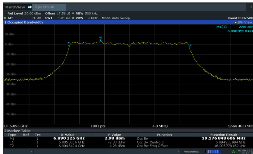
Fig.81 99% Occupied Bandwidth (802.11ax-HE20, 6895MHz)
