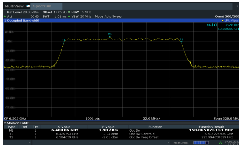
Fig.111 99% Occupied Bandwidth (802. 11ax-HE160, 6505MHz)
