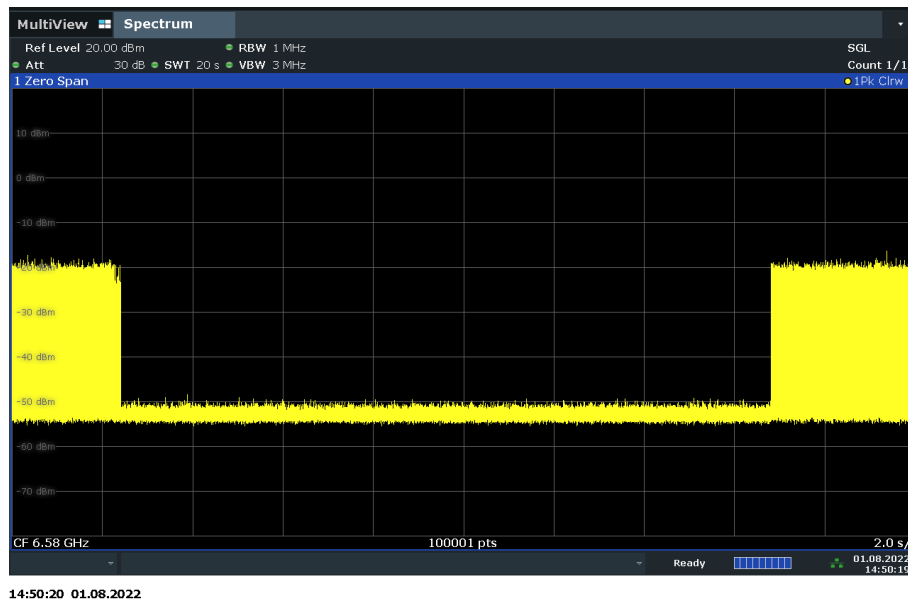
Fig.118 Contention Based Protocol 802.11ax HE160 (Upper edge ceased transmission)
