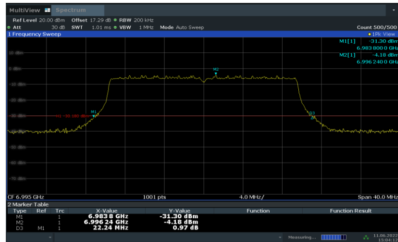
Fig.24 Occupied 26dB Bandwidth (802.11ax-HE20, 6895MHz)
