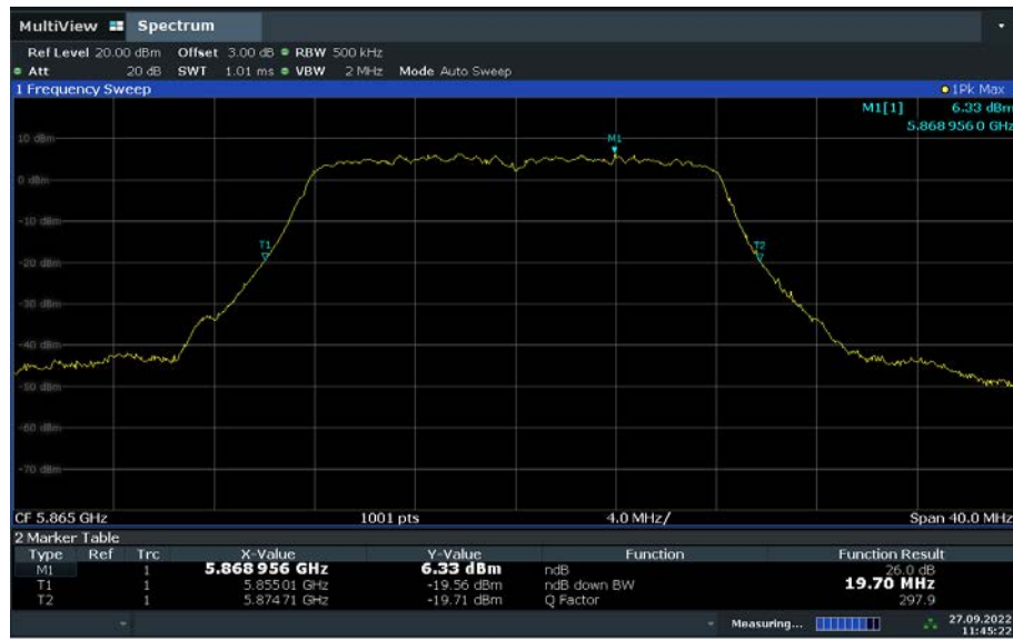
Fig. 78 Occupied 26dB Bandwidth (802.11a, channel 173)
