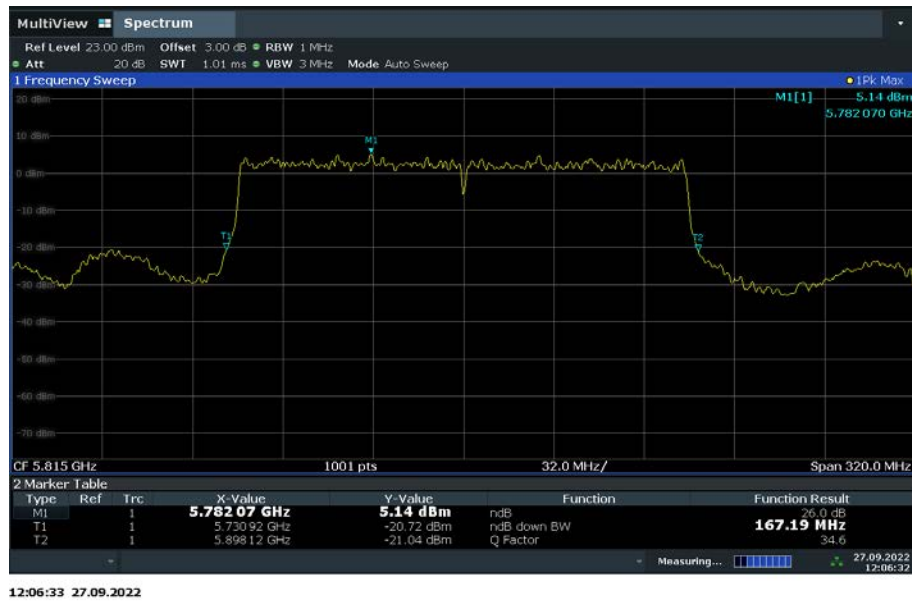
Fig. 86 Occupied 26dB Bandwidth (802.11ax-HE160, channel 163)
