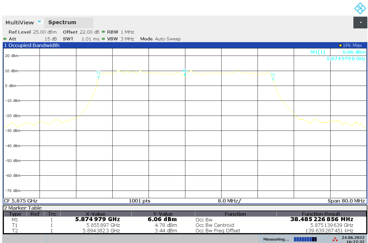
Fig. 18 99% Occupied Bandwidth (802.11ax-HE40, Ch 175)
