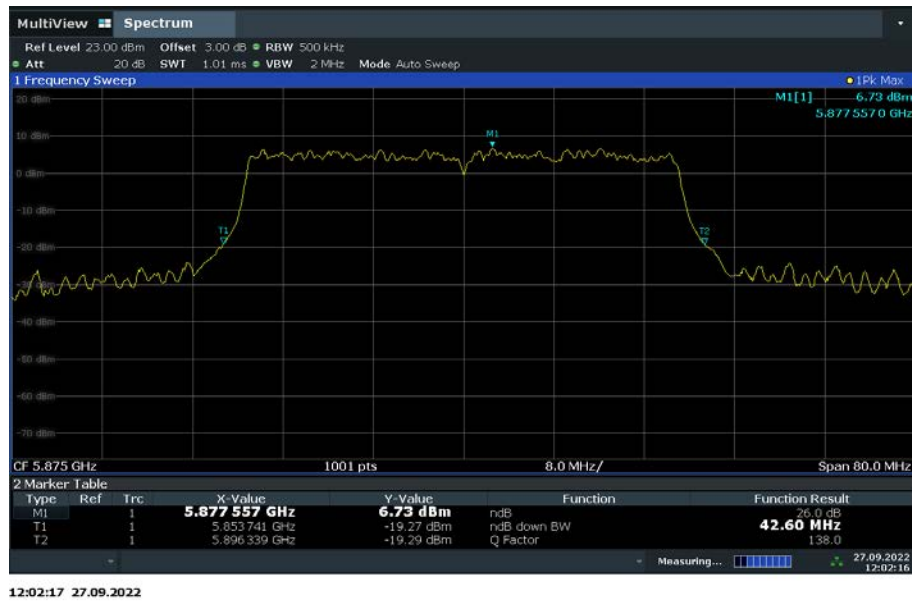
Fig. 84 Occupied 26dB Bandwidth (802.11ax-HE40, channel 175)
