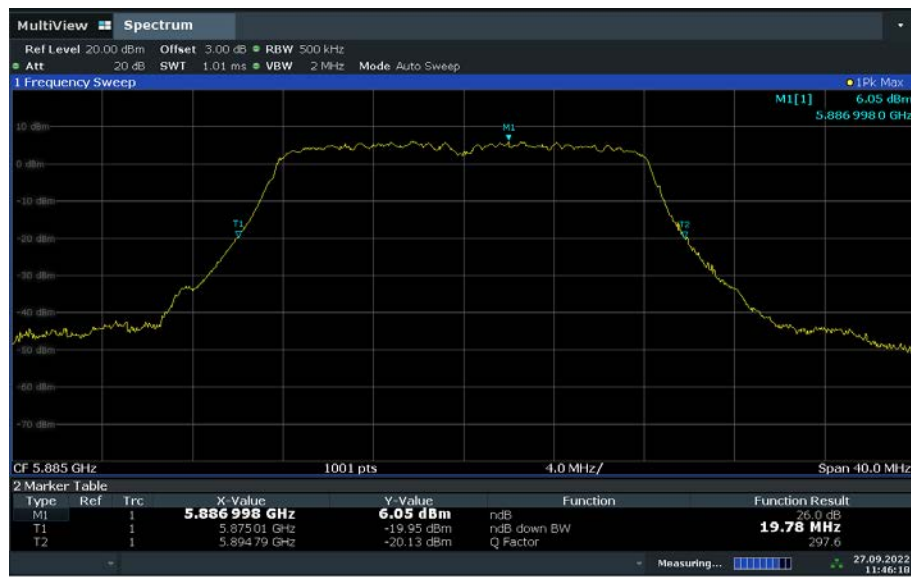
Fig. 79 Occupied 26dB Bandwidth (802.11a, channel 177)
