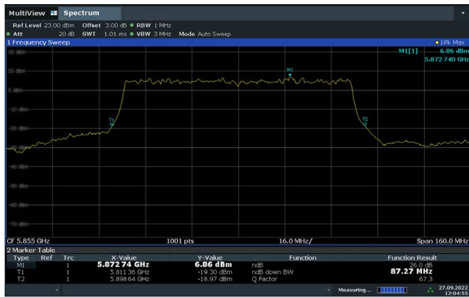
Fig. 85 Occupied 26dB Bandwidth (802.11ax-HE80, channel 171)
