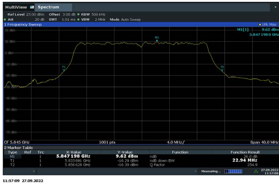
Fig. 80 Occupied 26dB Bandwidth (802.11ax-HE20, channel 169)
