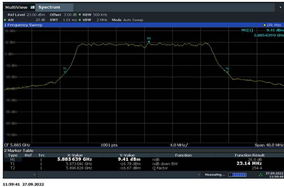
Fig. 82 Occupied 26dB Bandwidth (802.11ax-HE20, channel 177)
