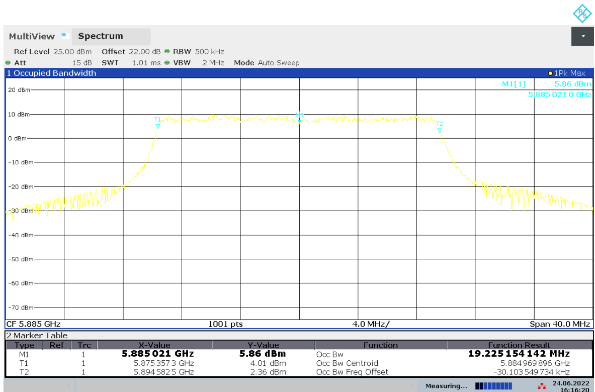
Fig. 16 99% Occupied Bandwidth (802.11ax-HE20, Ch 177)
