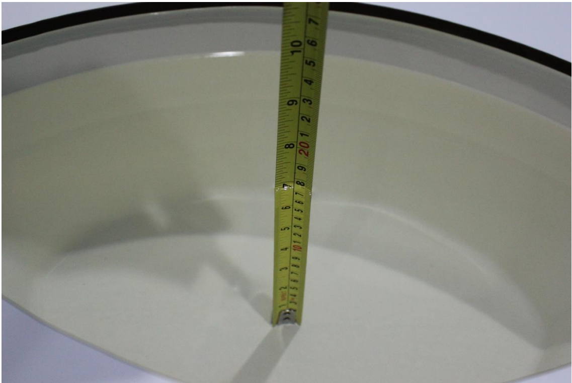
Picture 7- Liquid depth in the Head Phantom (5GHz)
