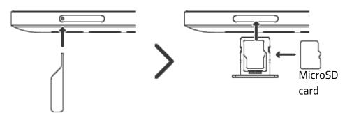
MicroSD card and ejector pin not included. Class 10 microSD card (up to 2TB) recommended.
