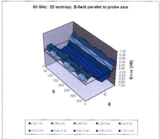
Probe isotropy for  $E_{tot}$ : probe rotated  $\phi=0^{\circ}$  to 360°, tilted from field propagation direction  $\overline{k}$  Parallel to the field propagation ( $\psi=0^{\circ}$  - 90°) at 30 GHz: deviation within  $\pm$  0.33 dB Parallel to the field propagation ( $\psi=0^{\circ}$  - 90°) at 60 GHz: deviation within  $\pm$  0.42 dB
