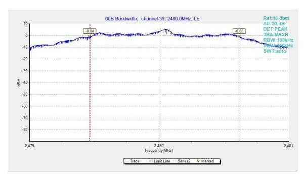
Fig.22. 6dB Bandwidth: GFSK, 2480 MHz
