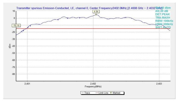
Fig.5. Transmitter Spurious Emission - Conducted: GFSK,2402MHz
