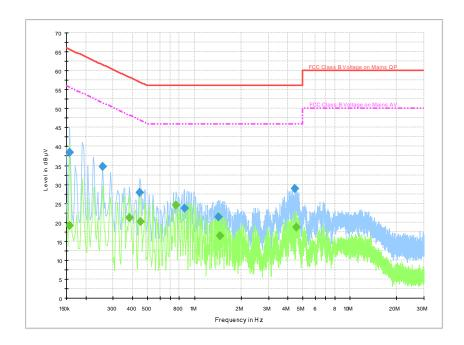
Fig.B.9.2 AC Powerline Conducted Emission-Idle
