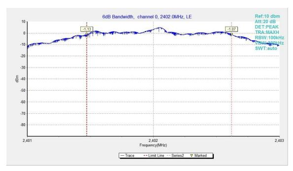
Fig.20. 6dB Bandwidth: GFSK, 2402 MHz
