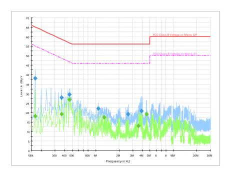
Fig.B.9.1 AC Powerline Conducted Emission- bluetooth
