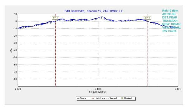
Fig.21. 6dB Bandwidth: GFSK, 2440 MHz
