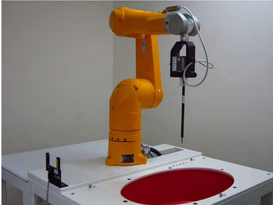
Fig.1 Photograph of the SAR measurement system
