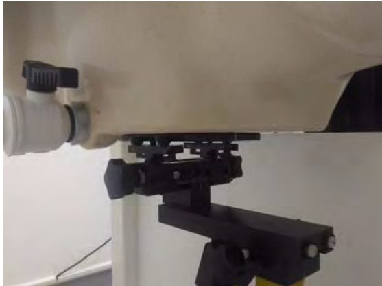
Fig.16 EUT Front side to flat phantom
