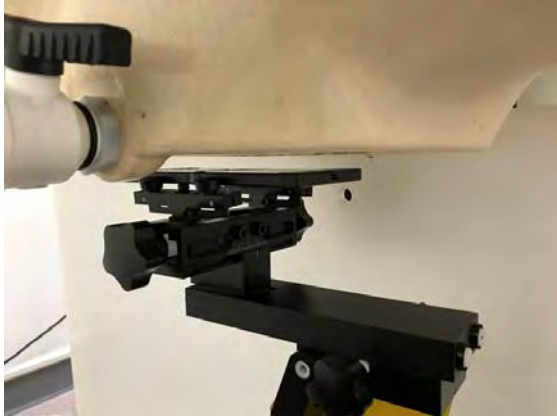
Fig.9 EUT Front side to flat phantom
