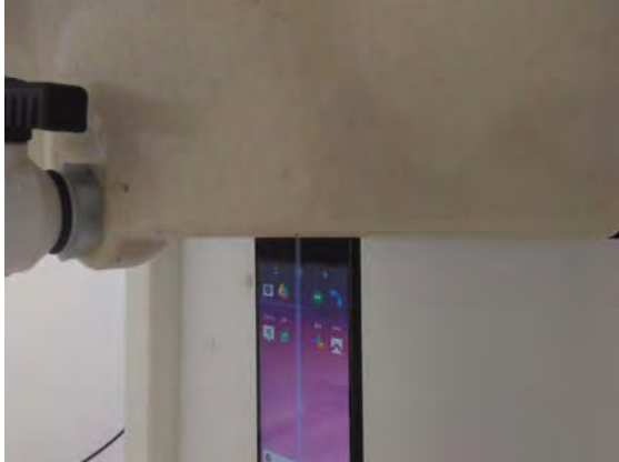
Fig.18 EUT Bottom side to flat phantom
