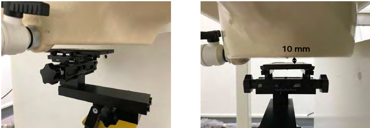
Fig.8 EUT Back side to flat phantom
