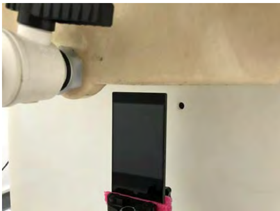
Fig.11 EUT Bottom side to flat phantom
