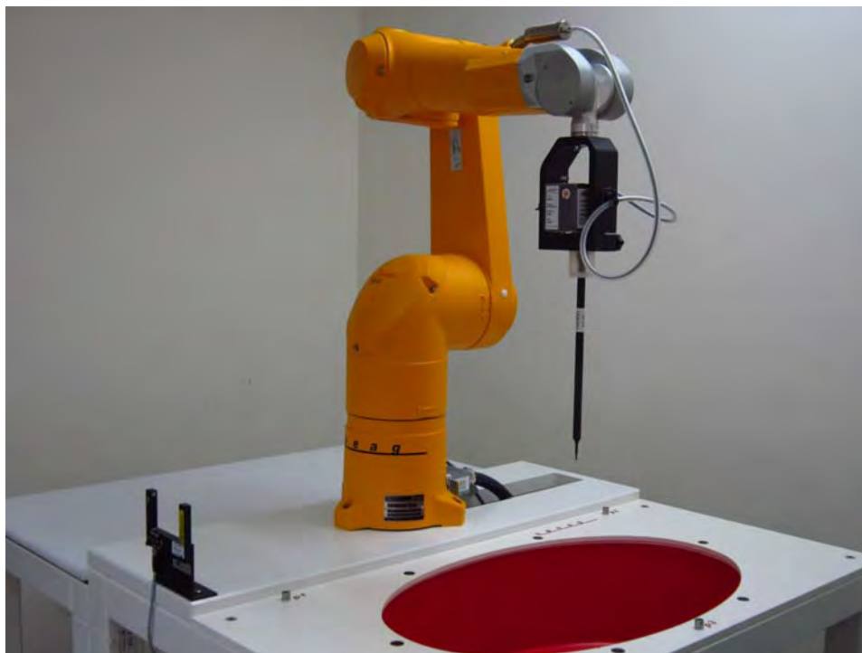
Fig.1 Photograph of the SAR measurement system
