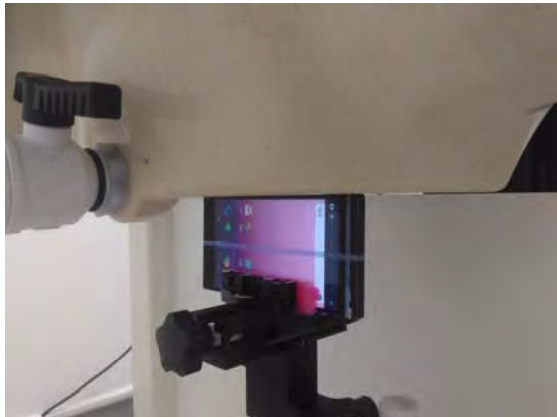
Fig.20 EUT Left side to flat phantom
