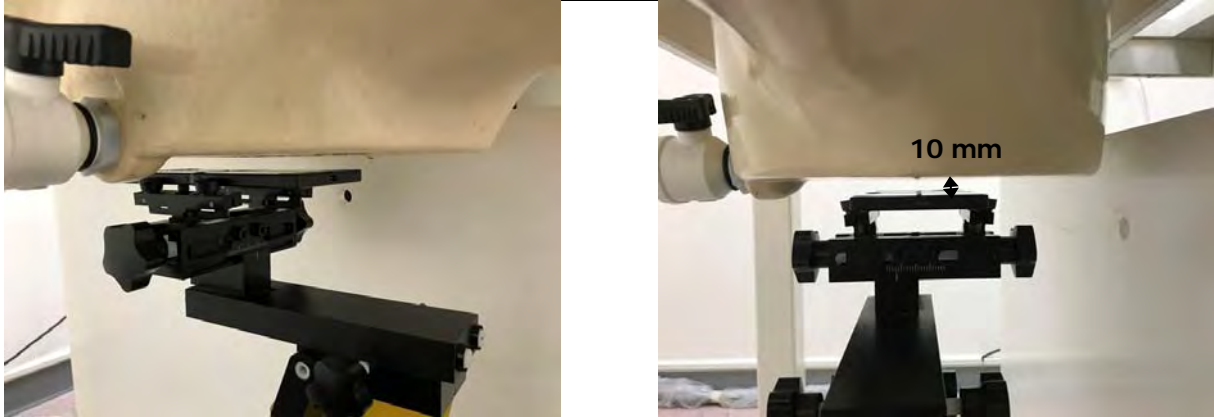
Fig.7 EUT Front side to flat phantom
