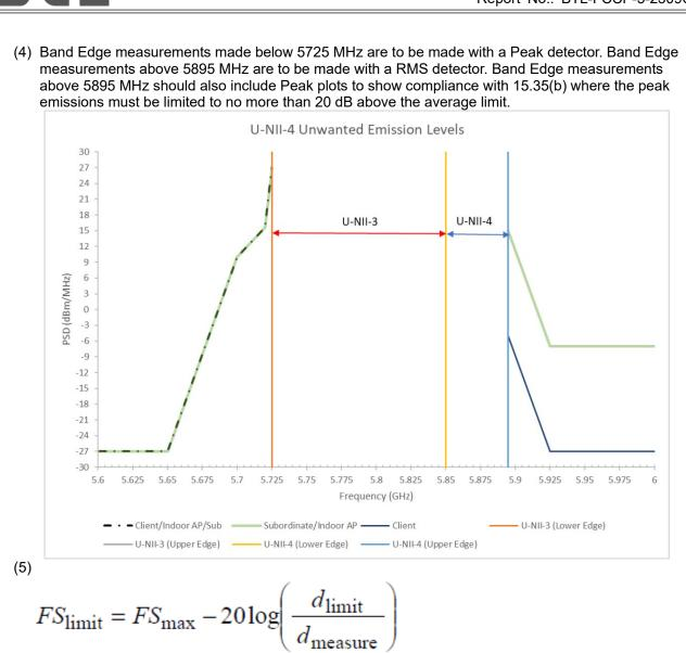
20log (d<sub>limit</sub>/d<sub>measure</sub>)=20log (3/1.5)=6 dB.
