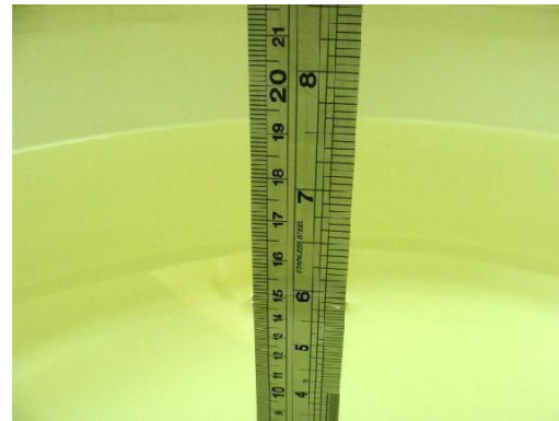
Fig 7.2 Photo of Liquid Height for Body SAR
