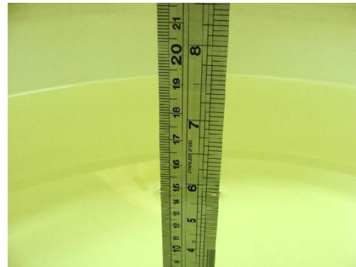
Fig 7.2 Photo of Liquid Height for Body SAR
