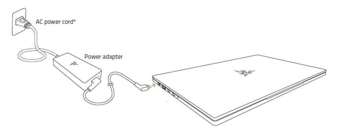
Make sure that the AC plug is properly inserted into the power outlet and the power adapter. Insert the power adapter's connector into the Razer Blade's power port. Press the power button to turn on your Razer Blade.
