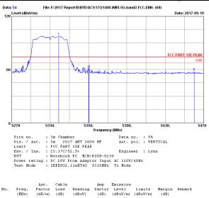
1 5319.00 33.23 2 5350.00 33.17 3 5350.60 33.17 4 5460.00 32.99 12.99 13.02 85.48 47.96 34.10 34.18 97.60 59.97 74.00 74.00 -23.60 14.03 Peak Peak 13.06 13.22 48.68 45.81 34.18 34.33 60.73 57.69 74.00 74.00 13.27 16.31 Peak Peak Remarks: 1. Emission Level= Antenna Factor + Cable Loss + Reading -Amp factor.
