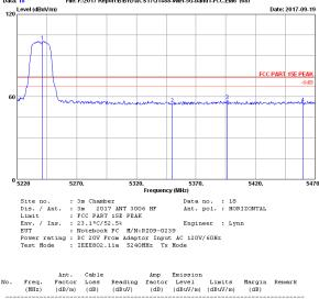
5241.25 33.38 5350.00 33.17 5396.25 33.08 5460.00 32.99 87.97 42.75 45.15 43.35 1 2 12.86 13.02 33.99 34.18 100.22 54.76 74.00 74.00 -26.22 Peak Peak 3 4 13.12 13.22 34.22 34.33 57.13 55.23 74.00 74.00 16.87 18.77 Peak Peak Remarks: 1. Emission Level= Antenna Factor + Cable Loss + Reading -Amp factor.
