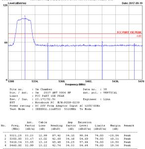
34.25 34.33 Remarks: 1. Emission Level= Antenna Factor + Cable Loss + Reading -Amp factor.
