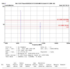
1 5180.00 33.47 2 10360.00 38.29 3 10360.00 38.29 12.76 18.14 18.14 90.03 28.50 41.40 33.91 102.35 35.58 49.35 35.58 62.25 74.00 -28.35 Peak 54.00 74.00 4.65 11.75 Average Peak Remarks: 1. Emission Level- Antenna Factor + Cable Loss + Reading -Amp factor.
