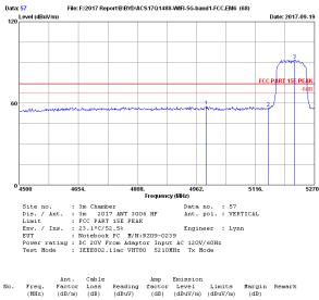
4987.41 33.80 5150.00 33.53 5217.64 33.41 45.23 43.99 79.75 74.00 74.00 74.00 12.42 12.69 33.66 33.87 57.79 56.34 16.21 17.66 33.95 12.83 92.04 -18.04 Peak Remarks: 1. Emission Level= Antenna Factor + Cable Loss + Reading -Amp factor. 2. The emission levels that are 20dB below the official limit are not reported.
