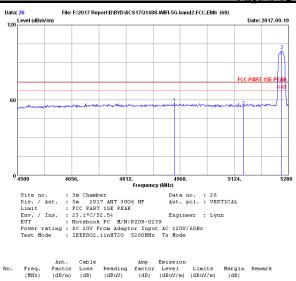
1 2 3 4952.40 5150.00 5260.50 33.70 33.53 33.32 45.24 42.63 87.41 74.00 74.00 74.00 16.37 19.02 -25.60 12.38 12.69 33.69 33.87 57.63 54.98 Peak Peak 12.89 34.02 99.60 Peak Remarks: 1. Emission Level= Antenna Factor + Cable Loss + Reading -Amp factor. 2. The emission levels that are 20dB below the official limit are not reported.
