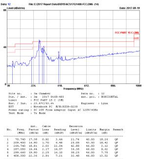
Remarks: 1. Emission Level= Antenna Factor + Cable Loss + Reading. 2. The emission levels that are 2048 below the official limit are not reported.
