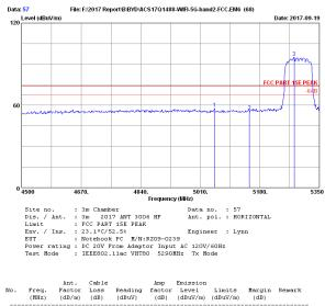
45.30 43.43 82.70 74.00 74.00 74.00 57.85 55.78 94.85 5050.80 33.71 33.53 12.56 12.69 33.72 33.87 16.15 18.22 5150.00 33.53 5277.75 33.29 12.92 -20.85 34.06 Peak Remarks: 1. Emission Level= Antenna Factor + Cable Loss + Reading -Amp factor. 2. The emission levels that are 20dB below the official limit are not reported.
