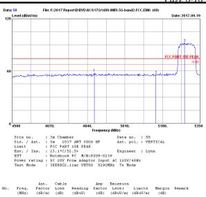
4871.45 5150.00 5280.30 33.56 33.53 33.29 46.20 43.32 80.36 74.00 74.00 74.00 1 2 3 12.22 33.75 33.87 58.23 55.67 15.77 18.33 Peak Peak 12.92 34.06 92.51 -18.51 Peak Remarks: 1. Emission Level= Antenna Factor + Cable Loss + Reading -Amp factor. 2. The emission levels that are 20dB below the official limit are not reported.
