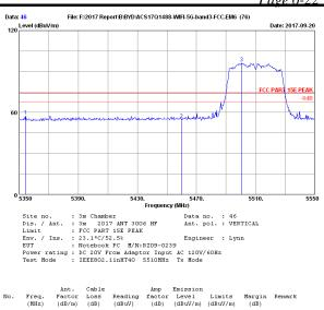
5354.40 5460.00 5500.60 33.17 32.99 32.90 45.40 42.97 84.38 34.18 34.33 34.37 74.00 74.00 74.00 1 2 3 13.06 13.22 57.45 54.85 16.55 19.15 Peak Peak 13.29 96.20 -22.20 Peak Remarks: 1. Emission Level= Antenna Factor + Cable Loss + Reading -Amp factor. 2. The emission levels that are 20dB below the official limit are not reported.
