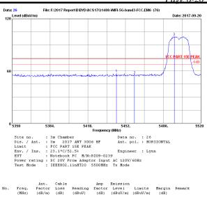
5443.84 5460.00 5495.86 33.02 32.99 32.93 34.29 34.33 34.37 74.00 74.00 74.00 1 2 3 16.37 18.67 -25.71 13.19 13.22 45.71 43.45 57.63 55.33 Peak Peak 13.29 87.86 99.71 Peak Remarks: 1. Emission Level= Antenna Factor + Cable Loss + Reading -Amp factor. 2. The emission levels that are 20dB below the official limit are not reported.
