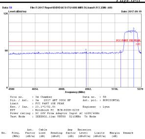
4950.45 33.70 5150.00 33.53 5225.34 33.38 46.08 43.44 80.75 33.69 33.87 33.99 74.00 74.00 74.00 15.53 18.21 -18.97 1 2 3 12.38 12.69 58.47 55.79 Peak Peak 12.83 92.97 Peak Remarks: 1. Emission Level= Antenna Factor + Cable Loss + Reading -Amp factor. 2. The emission levels that are 20dB below the official limit are not reported.
