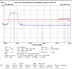
5233.40 33.38 5350.00 33.17 5447.04 32.99 5460.00 32.99 1 2 12.86 13.02 85.82 43.13 33.99 34.18 98.07 55.14 74.00 74.00 -24.07 Peak Peak 3 4 74.00 13.19 13.22 46.50 43.41 34.29 34.33 58.39 55.29 15.61 18.71 Peak Peak Remarks: 1. Emission Level= Antenna Factor + Cable Loss + Reading -Amp factor.
