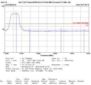
5322.95 33.23 5350.00 33.17 5413.39 33.05 5460.00 32.99 1 2 3 4 12.99 13.02 88.80 43.47 34.14 34.18 100.88 55.48 74.00 74.00 -26.88 18.52 Peak Peak 45.33 43.46 13.16 13.22 34.25 34.33 57.29 55.34 74.00 74.00 16.71 18.66 Peak Peak Remarks: 1. Emission Level= Antenna Factor + Cable Loss + Reading -Amp factor.
