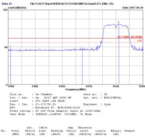
45.78 43.27 85.74 34.18 34.33 34.45 74.00 74.00 74.00 5353.60 33.17 32.99 13.06 13.22 57.83 55.15 16.17 18.85 1 5460.00 5514.00 32.92 -23.50 13.29 97.50 Peak Remarks: 1. Emission Level= Antenna Factor + Cable Loss + Reading -Amp factor. 2. The emission levels that are 20dB below the official limit are not reported.
