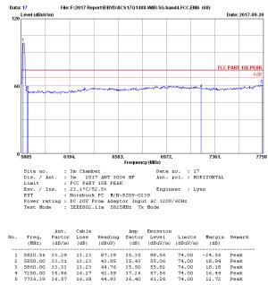
16.27 16.18 Remarks: 1. Emission Level\* Antenna Factor + Cable Loss + Reading -Amp factor.
