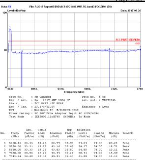
43.83 43.44 45.51 Peak Peak Peak Peak 16.27 16.18 37.26 36.40 58.41 61.89 74.00 74.00 Remarks: 1. Emission Level= Antenna Factor + Cable Loss + Reading -kmp factor.
