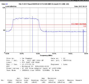
1 5309.68 33.23 2 5350.00 33.17 3 5459.68 32.99 4 5460.00 32.99 12.96 13.02 81.12 44.15 34.10 34.18 93.21 56.16 74.00 74.00 -19.21 17.84 Peak Peak 45.85 44.81 13.22 13.22 34.33 34.33 57.73 56.69 74.00 74.00 16.27 17.31 Peak Peak Remarks: 1. Emission Level= Antenna Factor + Cable Loss + Reading -Amp factor.
