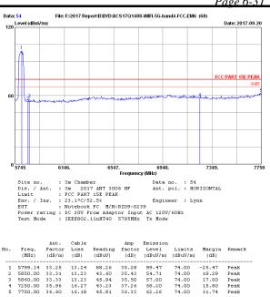
37.26 36.33 Remarks: 1. Emission Level= Antenna Factor + Cable Loss + Reading -kmp factor.
