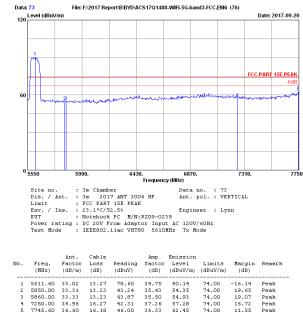
Remarks: 1. Emission Level= Antenna Factor + Cable Loss + Reading -Amp factor.
