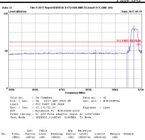
4975.96 5150.00 5186.20 33.77 33.53 33.47 12.42 12.69 12.76 74.00 74.00 74.00 16.37 18.11 -22.44 1 2 3 45.10 43.54 33.66 33.87 57.63 55.89 Peak Peak 84.12 33.91 96.44 Peak Remarks: 1. Emission Level= Antenna Factor + Cable Loss + Reading -Amp factor. 2. The emission levels that are 20dB below the official limit are not reported.
