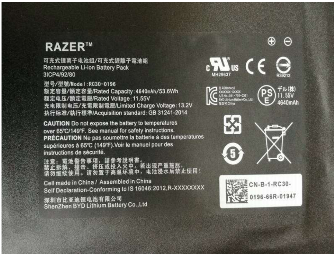
Figure 19 Label of Battery
